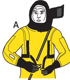
**B.** While squatting, grab face flap (red tab) and pull forward to release excess air from the suit (1). Secure face flap over face or off the face by matching hook and loop fasteners (2).
