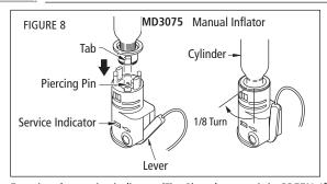
5) Examine the service indicator (Fig. 8) and ensure it is GREEN. If the service indicator is red, the mechanism has been fired or is incorrectly fitted and the inflator requires service. See Re-arming Your PFD (MD3075) p. 6.
