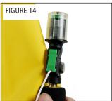
Step 4 - Check to be sure service indicator is green inside clear cap and the green indicator clip is firmly attached to the activation lever (Fig. 14).
