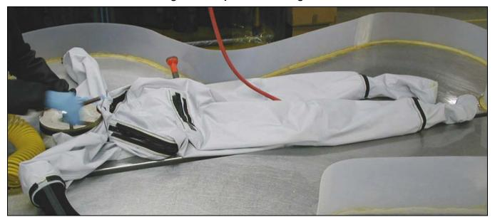
b. Carefully seal the wrists of the suit with suitable clamps.
